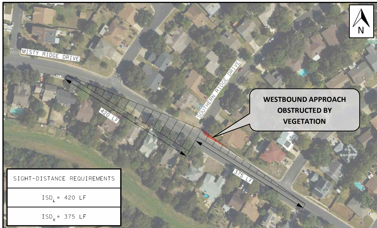
Figure 36 – Sight Distance Analysis: Southbound Southern Ridge Drive at Misty Ridge Drive
